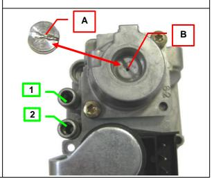
Note: The VK41 gas valve block is to be replaced to switch from the second-family gases, adjustable from 1.5 to 20 mbar, to the third-family gases, adjustable from 37 to 50 mbar.
