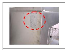
Position of the data plate on V02228-V02683
