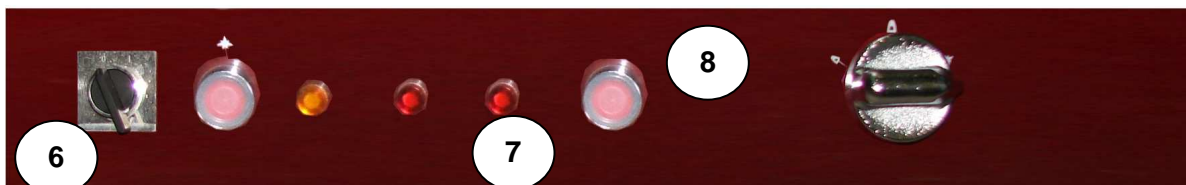
Bratt pan with ignition and manual safety reset
