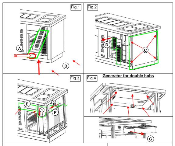
1) Unscrew the front panel (A) (fig.1). Pull it. Lift it.
