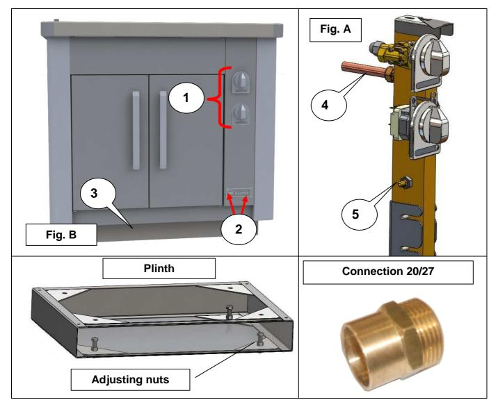
Remove the control knobs, ((1) screwed).
